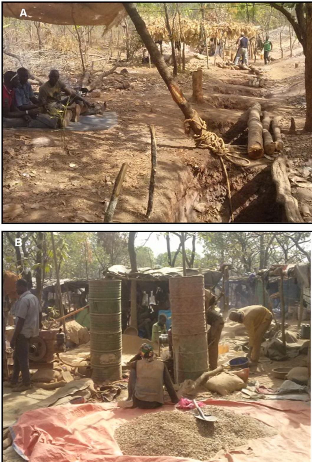
FIGURE 8.1: (A) Kehi 2015 Artisanal pits with ore hoisting mechanism and (B) Crushing and processing of the gold bearing gravels.
